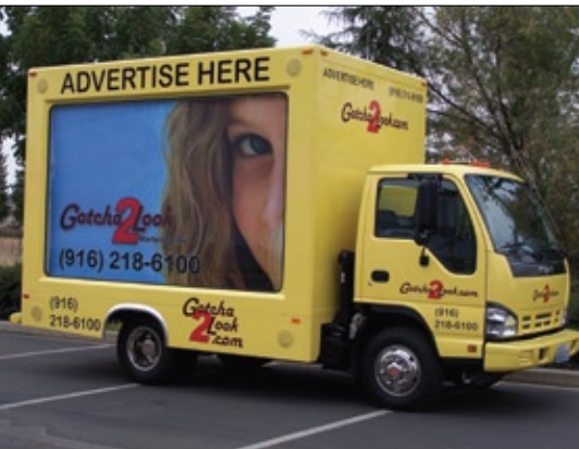
This Isuzu NPR medium-duty diesel truck used by Gotcha2Look Marketing Inc. in Sacramento, Calif., used a B-20 blend of biodiesel (20 percent biodiesel/80 percent petroleum diesel) without any difference in performance characteristics compared to regular diesel.
